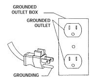
plugged into an appropriate outlet that is properly installed and grounded in accordance with all local codes and ordinances.
